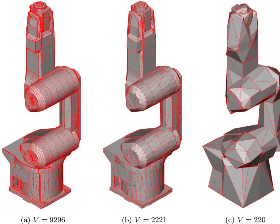
Figure 1: Complex meshes (a) are simplified effectively by our new bounding mesh (b) and bounding sets convex polyhedra (c) algorithms.
