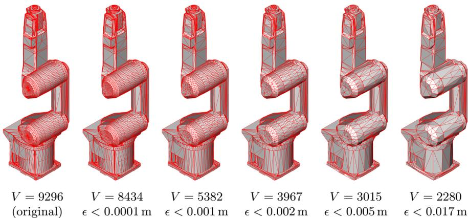
Figure 4: A series of bounding meshes tightly approximates a ROBOT geometry by enclosing meshes, greatly reducing the number of vertices.
