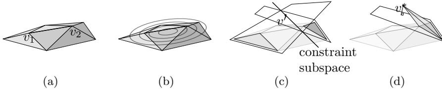
Figure 2: Bounded edge contraction. (a) Edge with neighboring planes, (b) quadric cost matrix  $Q$ , (c) example of a case  $m = 2$  minimizer, (d) global constraint minimizer  $v^*$  adds tetrahedron volumes on each plane that have positive heights
