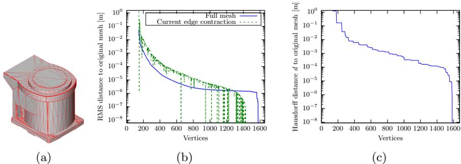
Figure 3: ROBOT BASE: Bounding mesh precision with respect to vertex count. (a) Original mesh, (b) quadric cost function  $E$  with respect to vertex count, (c) exact Hausdorff distance  $d$  to original mesh
